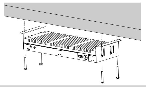
Wall mounting (ventilation slots heat sink vertical and facing away from the wall)
